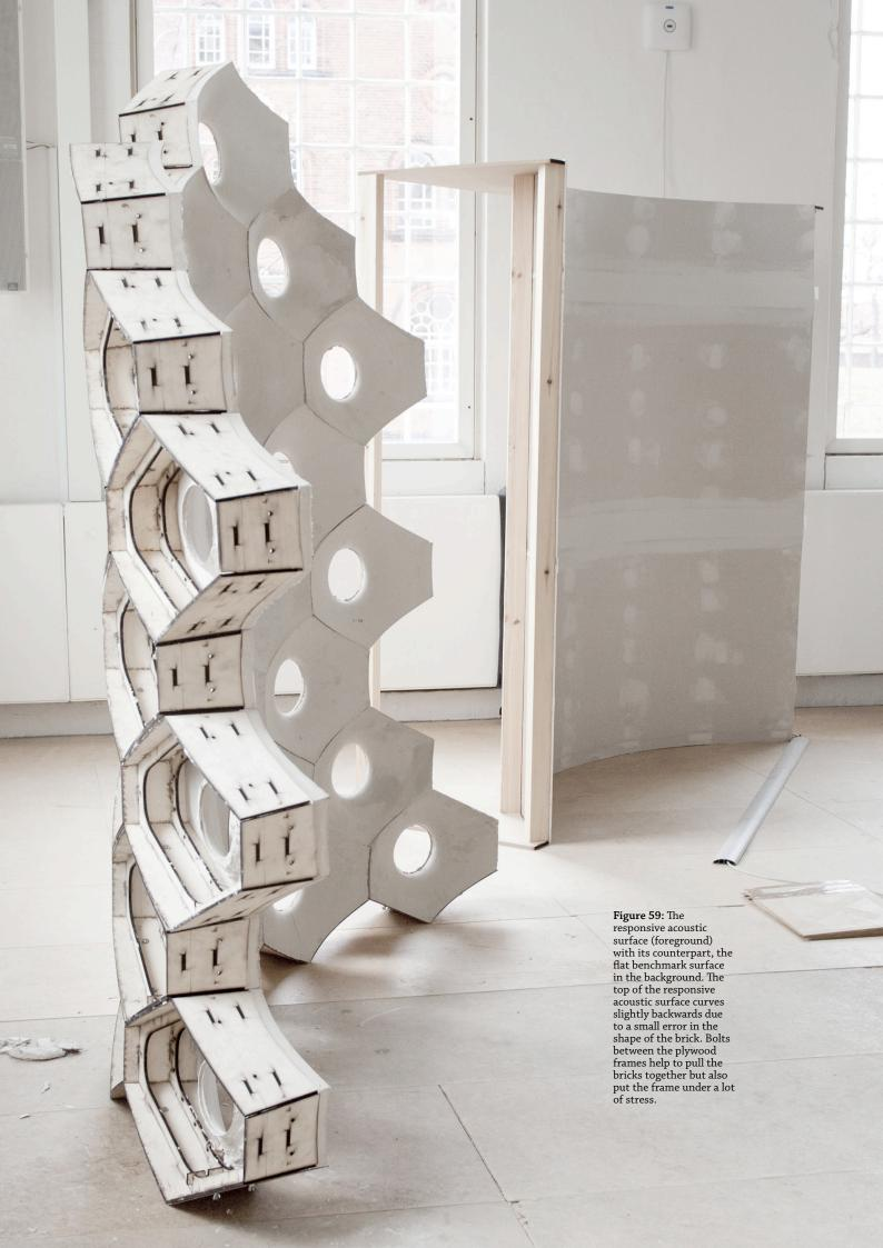
error threatened the whole viability of the project. Once again we were without sleep. Thankfully the timber formwork had enough pliability to accommodate the error, although if you look closely at figure 59 you can see the timber is under such tension the whole wall bows slightly backwards.
